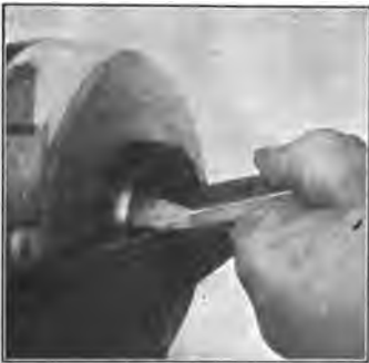
Fig. 171. Skew Chisel Smoothing Ring.
